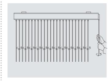
If any slats are misaligned, rotate the wand until the slats are fully closed. Continue twisting until all slats are aligned correctly.
