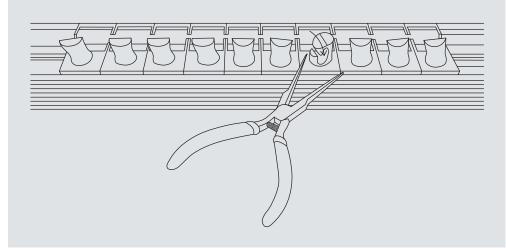
Did this align all the pegs? If not, gently rotate the lazy traveller with a pair of pliers. The traveller will then click into place accordingly.
