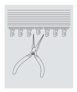
If not, check if any of the pegs within the headrail have been pushed in, if they have, using a pair of pliers, gently pull the pegs back out.
