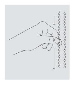
Repeat step 2 pulling chain in the opposite direction until travellers are fully aligned.
